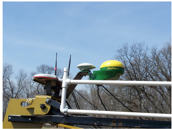
Figure 5: Mounting of Leica RTK GPS antenna. Other antennas were not used in the data presented here.
