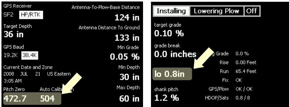
Figure 4: A low Pitch Zero will cause the plow to run too deep (too low).
