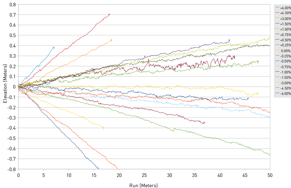
Figure 3: Plow installation profiles when operated at various pitches
